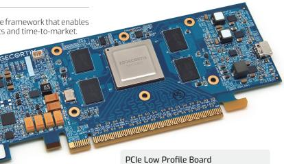
EdgeCortix SAKURA-I is available on a PCIe Low Profile board, ready to drop into a host for software development and AI model inference tasks.
