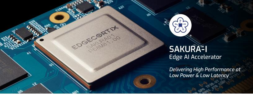
EdgeCortix SAKURA-I is a TSMC 12nm FinFET co-processor (accelerator) delivering efficient compute and low latency for edge artificial intelligence (AI) inference. It is powered by a 40 TOPS (dense), single core Dynamic Neural Accelerator® (DNA), which is EdgeCortix's proprietary neural processing engine with built-in runtime reconfigurable data-path effectively connecting all compute engines together.
