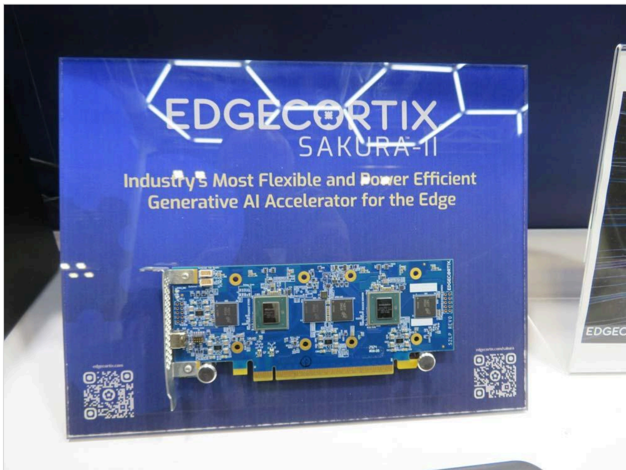
An accelerator PCIe card implementing 'SAKURA-II'
