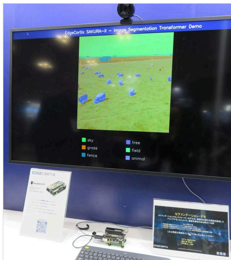
Demonstration of image segmentation with Generative AI on a Raspberry Pi
