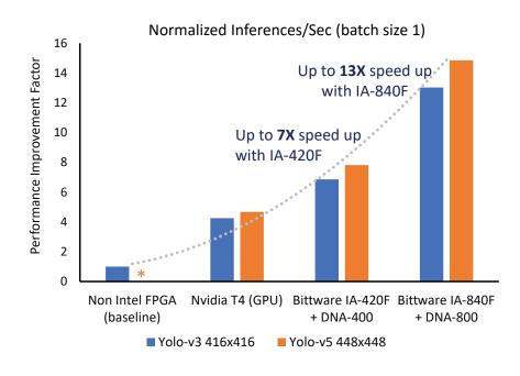
Comparing the inference performance of Edgecortix DNA running on BittWare cards with Intel Agilex FPGAs with the baseline of native Al acceleration IP on non-Intel FPGA and Nvidia T4 GPU, for state-of-the-art object detection models. Baseline of Yolov3 uses a solution that runs at 333 MHz on the non-Intel FPGA. DNA-400 and DNA-800 are new Intel Agilex optimized IP from EdgeCortix running at 350 MHz.
